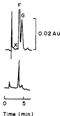
Figure 3. Chromatograms of reducing sugars in an extract from freeze-dried chicory root. In addition to fructose (F) and glucose (G), traces of xylose (X) and an unidentified component eluting after glucose appear in the upper chromatogram. Chromatographic conditions as in Figure 1. Detector range 0.128 AUFS (lower chromatogram) and 0.032 AUFS (upper chromatogram).
